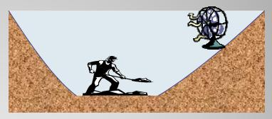
Elimination of the hazard is always the first priority. Good ventilation can eliminate an H<sub>2</sub>S hazard.
